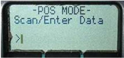
The POS Mode sends all scanned values to the computer as if they were entered through the keyboard. The **POS Mode** simply "types" the value on the keyboard. For example: if Notepad is open, whatever values are scanned will be typed into Notepad. Make sure the user is near the terminal to which the scanner base is connected before scanning in the **POS Mode**.
