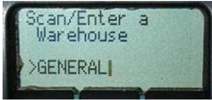
2. Type in the Warehouse name, or scan a barcode. A single beep and a green light mean that the entry is valid. An error sound (4 beeps) and a red light indicate that the warehouse was not entered properly.
