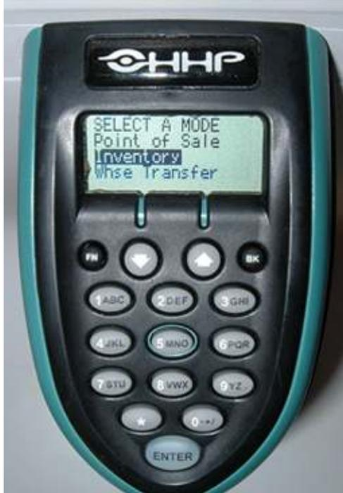
This is the menu which allows the user to select the mode to work in. The modes are as follows:
