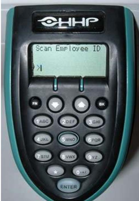
Scan or type in an employee ID. The employee ID's are found by going to **EBMS>Payroll>Employees**. If the ID is valid the scanner will beep once and the prompt will change. If the employee ID is invalid, the scanner will make an error sound. If the EBMS Timecard module is used by the company, the timecard login can be used as well.
